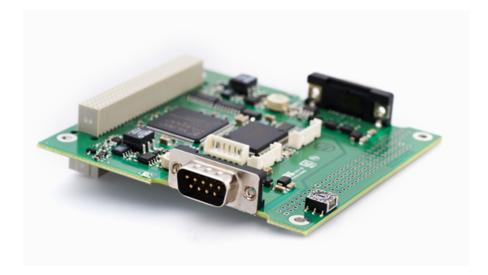
Kvaser PCI104 is a two channel, PCI-104 compatible CAN interface. It includes a high-performance, on-board microcontroller for CPU offloading, ensuring fast response times..
