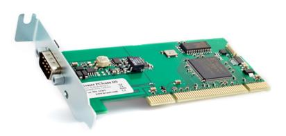
Kvaser PCIcanx is a high speed CAN interface for the PCI-X and PCI bus. It features Galvanic Isolation for protection against voltage spikes.
